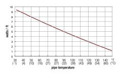
The Power Output Curve illustrates the relationship between wattage output and pipe temperature. As the pipe temperature rises, the heating cable uses less wattage and emits less heat.
